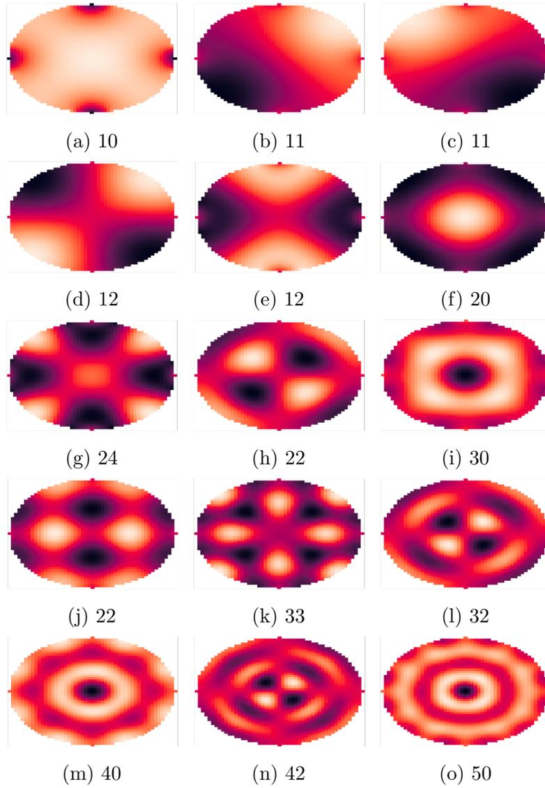
Figure 5: Field plots of (5x5) circular metal waveguide (2000 points, 3800 Mesh Elements)
