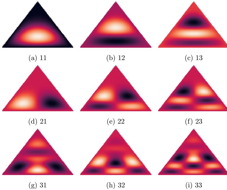
Figure 4: Field plots of (base:10, height:5) isosceles triangular metal waveguide (1700 points, 3200 Mesh Elements)
