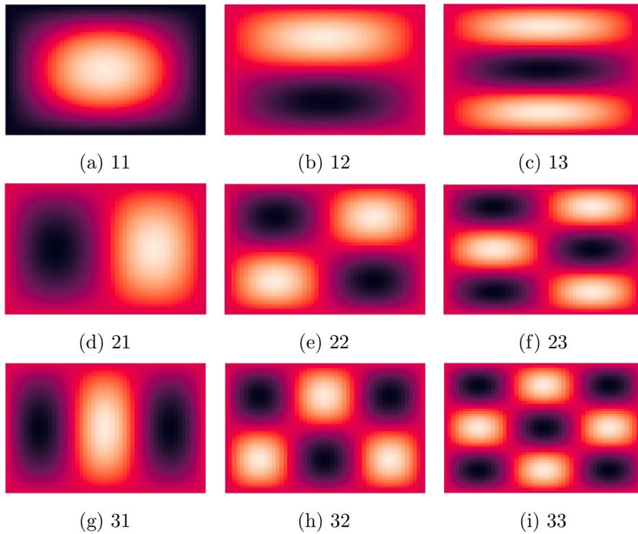
Figure 2: Field plots of (20x10) rectangular metal waveguide
