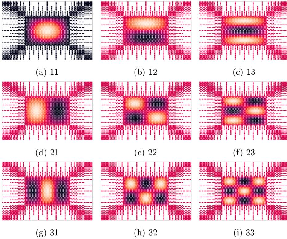
Figure 3: Field plots of (20x10) rectangular waveguide with a step index, placed in pseudo-infinite medium (3700 points, 7300 Mesh Elements)
